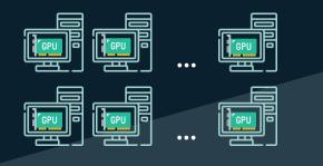
Workstations and GPUs in the traditional deployment model are configured on a 1:1 basis, having a dedicated GPU installed, and depending on chassis size, a limited number of supported GPUs. Additionally, power requirements and heat generation must be considered.
